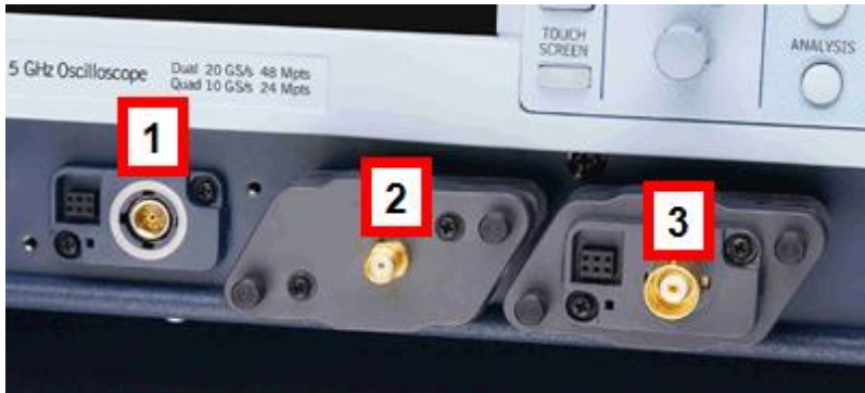
Figure 1-5. BMA Female Connector (1), ProLink BMA-to-SMA Adapter (Installed, 2), and ProLink BMA-to-BNC Adapter (Installed, 3)
