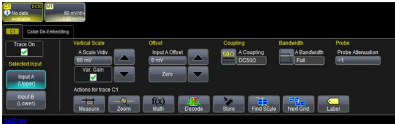
Figure 1-2. The channel screen layout showing Input A's ProLink interface controls setup
