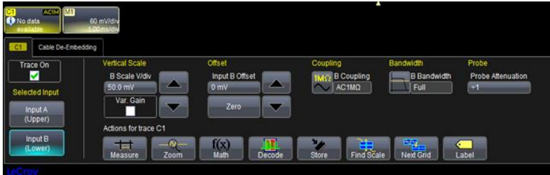
Figure 1-3. The channel screen layout showing Input B's ProBus interface controls setup
